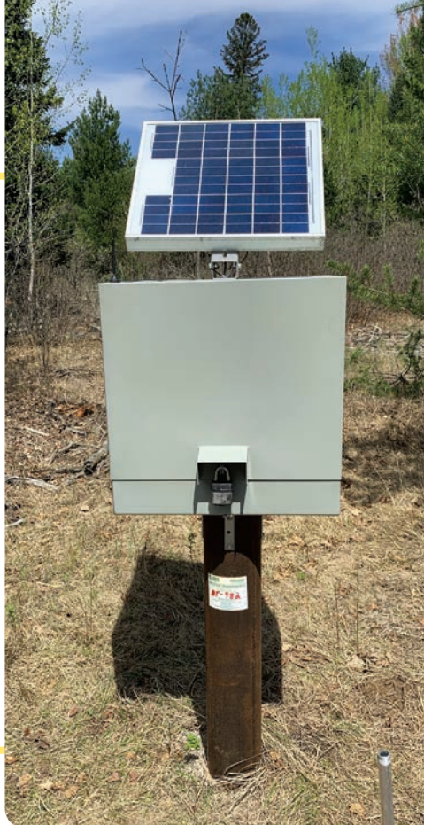
Well SC-0982 in Burnett County has an automatic logger connected to a cellular signal, allowing the data to be transmitted in real-time to the web. The site is powered by a solar panel.
